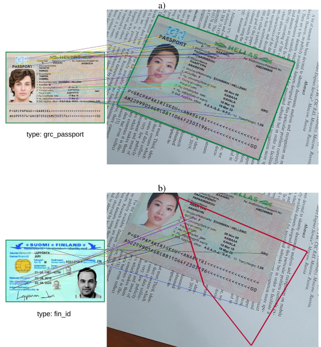
FIGURE 5. Example of correctly identified document type for MIDV-2020/photo grc_passport/28: matching with a) correct document type (grc_passport) and b) incorrect document type (fin_id). Inliers drawn. Localization result is illustrated by green quadrilateral ( D = 24.52, IoU = 0.98 ). For clarity, in case of incorrect document type here we also presented quadrilateral obtained by corresponding homography ( D = 1762.84, IoU = 0.32 ).
