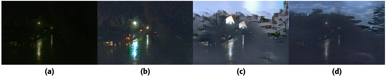
FIGURE 7. Style transfer and data augmentation methods with from left to right: Fig. 7a The input image, Fig. 7b CoMoGAN [38], Fig. 7c ManiFest [39], Fig. 7d MUNIT [21] trained on the Waymo dataset. These style transfer methods do not preserve the integrity of the scene in the input image and add hallucinations.
