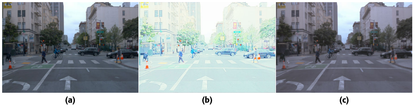
FIGURE 8. From left column to right column: the input normal-light image, the extracted raw illumination and the reflectance. Textural details such as the frontage of the buildings end up in the reflectance which demonstrates the quality of the decomposition model.
