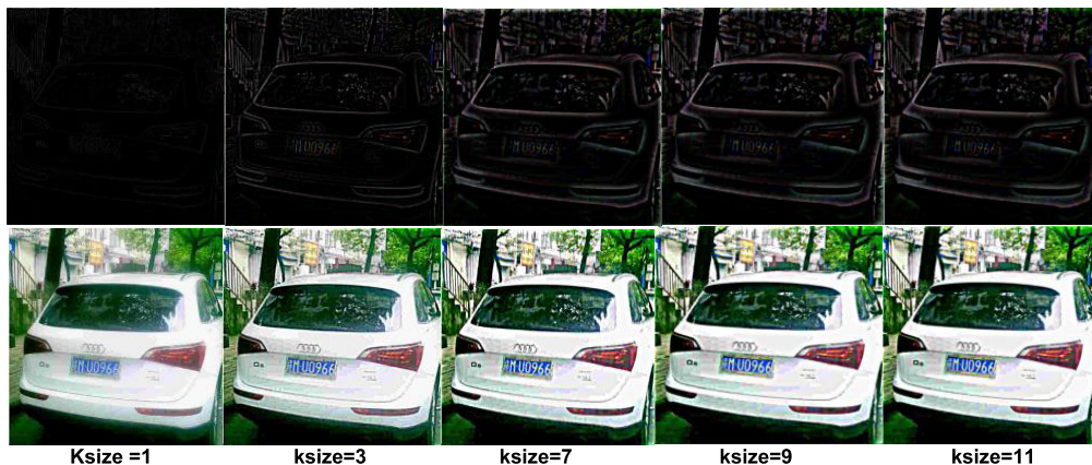
FIGURE 7. The experimental results of our approach in different Gaussian kernel sizes (ksizes), the first row is the original image, the second row is the extracted image details, and the last row is the detail-boostered image.
