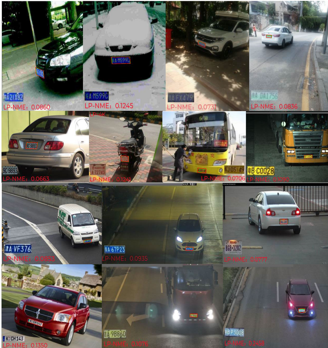
FIGURE 11. Partial samples of images, featuring a diverse range of objects. The first two images in the top row are sourced from the CCPD dataset, while the remaining images are sourced from the LPDE-4K dataset. The red box in each image represents the object detection result, while the green box indicates the ground truth bounding box. The corrected values of the LP and LP-NME metrics are displayed in the lower left corner of each image.
