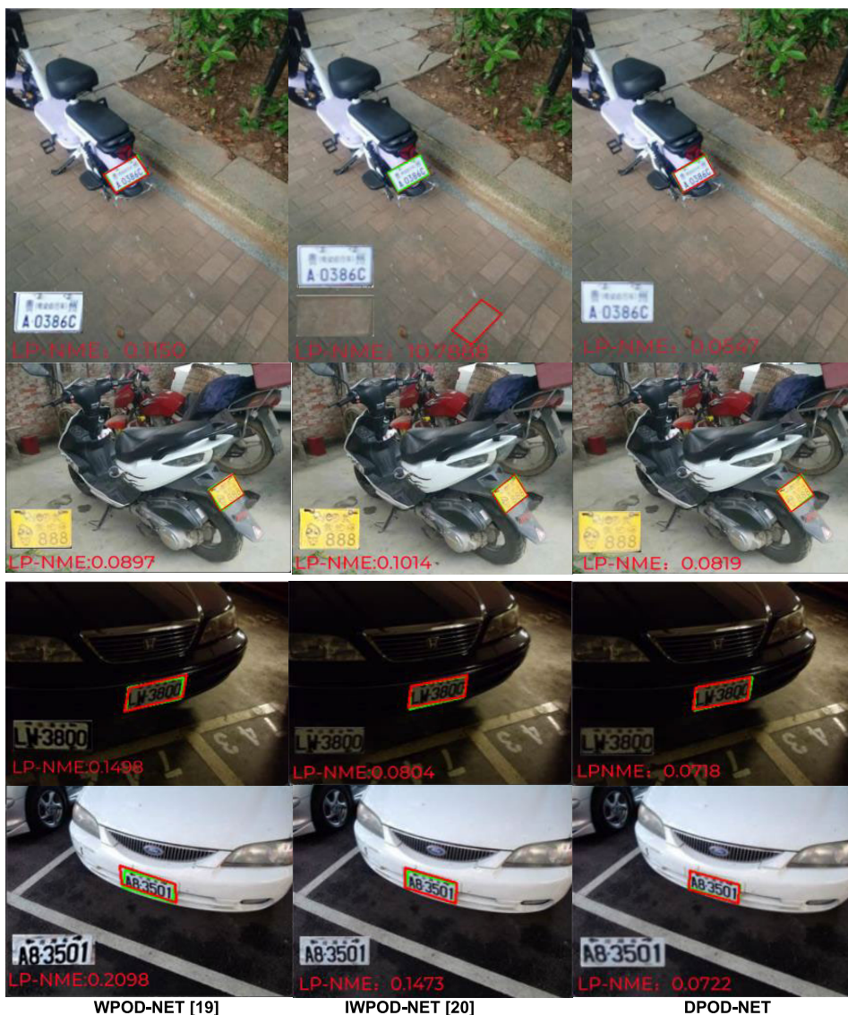
FIGURE 10. comparison of our approach with WPOD-NET [19] and IWPOD-NET [20], the red box represents the detection result, while the green box indicates the actual box. The corrected LP and LP-NME values can be found in the lower left corner of the each image. The images used in this comparison are from the LPDE-4K and ALOP datasets.
