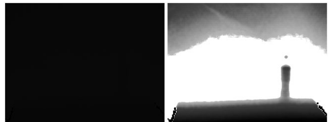
FIGURE 21. A comparative display of the original (left) and equalised (right) version of image 18 from the VDT-2048 dataset. The stark contrast between the two images accentuates the pivotal role of pre-processing in enhancing feature visibility, a critical step for the effective application of convolutional neural networks.
