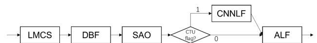
FIGURE 14. Pipeline of LDSCA. L: LMCS. D: DBF. S: SAO. C: CNNLF. A: ALF.
