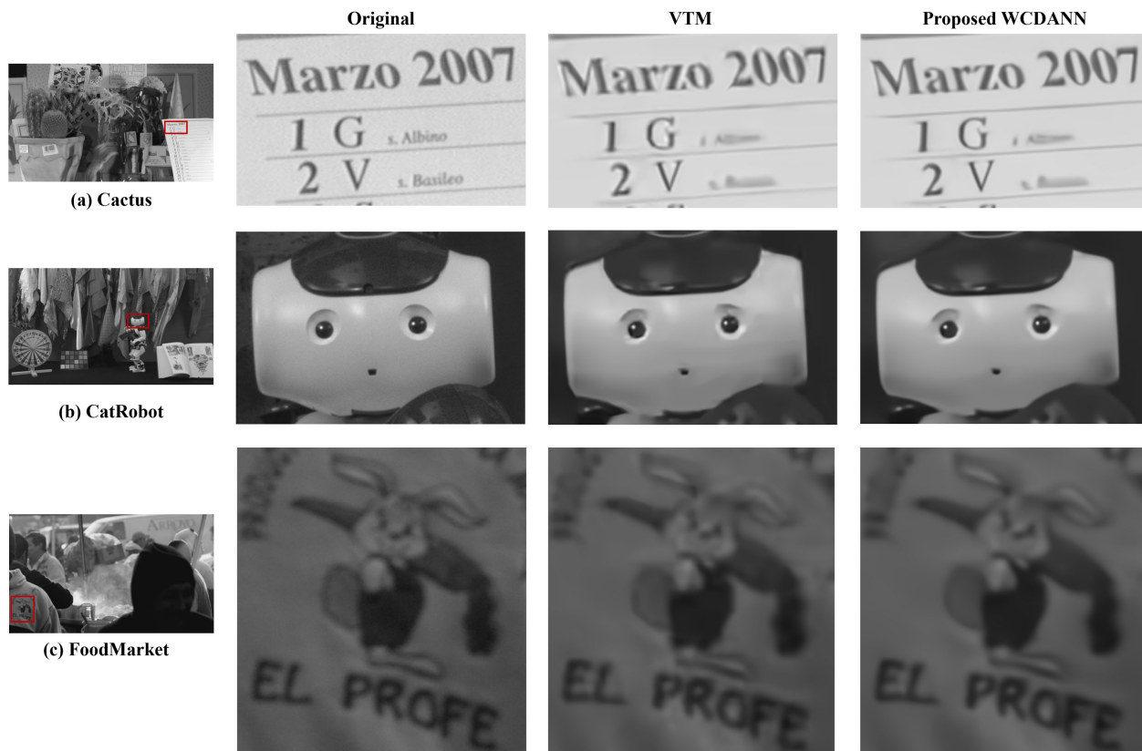
FIGURE 12. Comparison of visual quality between VTM-11.0-NNVC and WCDANN. (a) Class B-Cactus (QP=42, RA). (b) Class A2-CatRobot (QP=42, LDP). (c) Class A1-FoodMarket (QP=42, AI).
