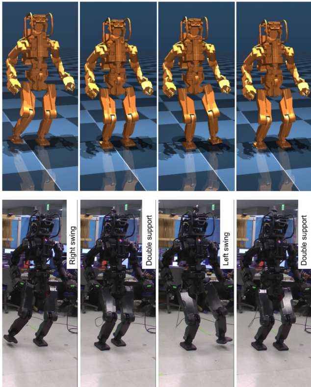
FIGURE 1. HRP-5P humanoid robot trained to perform bipedal locomotion via model-free reinforcement learning in MuJoCo (top); RL policy transferred to the real robot (bottom). We make use of the feedback from measured actuator current to account for the poor torque-tracking on the real system.
