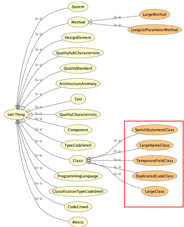
FIGURE 1. Classes of the ontology to represent code smells.
