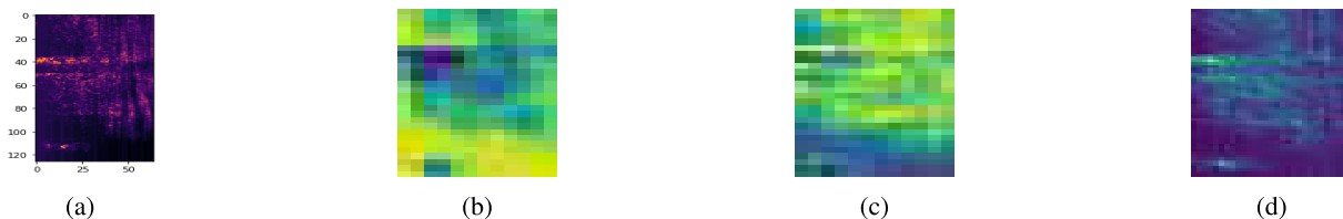
FIGURE 8. Phonotrauma: input "image" along with three feature activation maps of the final convolutional layer.
