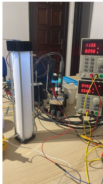
FIGURE 2. An example of an UV-LED disinfection module; in-lab tests.
