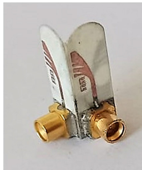
FIGURE 9. Fabricated prototype of the dual-polarized Vivaldi antenna.
