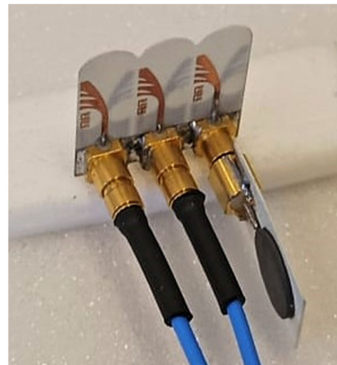
FIGURE 13. Fabricated prototype of the 3-element Vivaldi antenna array.
