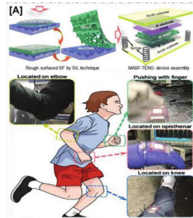
FIGURE 10. Flexible AT-MASF-TENG device to sense various human activities by locating it on different places of the body, i.e., under the finger, on the elbow, opisthenar of hand, and knee, respectively [67].
