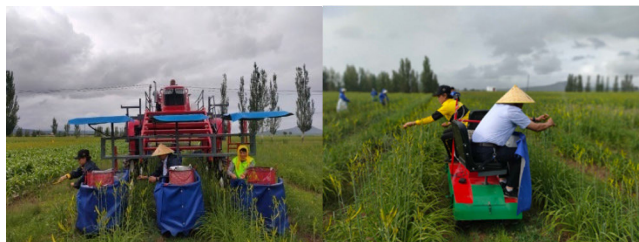
FIGURE 1. The 4HF-6 hanging (left) and 4HF-2 crawling (right) auxiliary daylily harvesters developed by our research team.
