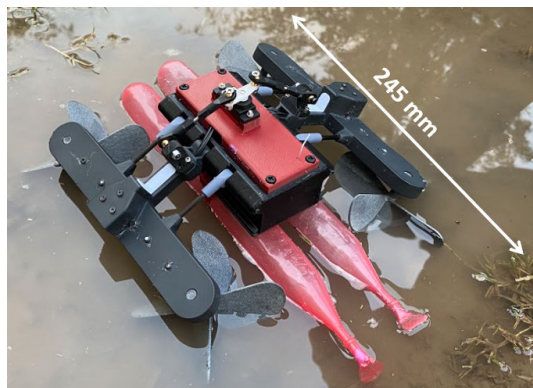
FIGURE 1. The AmphiSTAR is a newly developed STAR robot fitted with a sprawling mechanism and four propellers at its bottom. The two propellers at each side are actuated using a single brushless motor. The robot can crawl over the ground or swim and hover over water.
