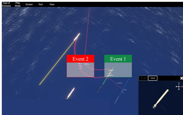
FIGURE 15. DVES screenshot of engagement procedure using multiple wire-guided torpedoes.
