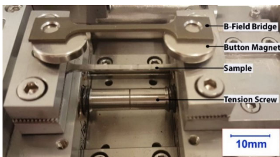
FIGURE 6. Sample and B-Field bridge orientation within the deben 5kN material miniature tensile tester.
