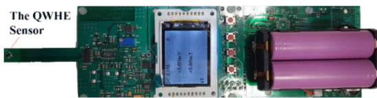
FIGURE 4. QWHE sensor based magnetometer, designed and developed at the university of manchester, used in the research.
