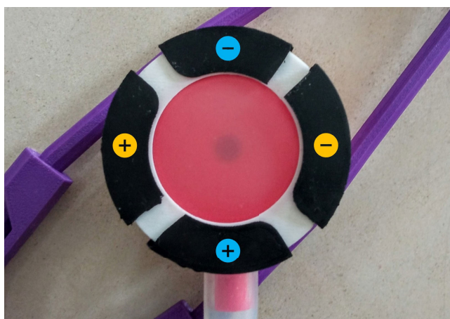
FIGURE 14. Disposition and polarity of two pairs of ECG dry electrodes on the stethoscope head, for the acquisition of two ECG leads. The electrodes with positive polarity are on the bottom and left sides.
