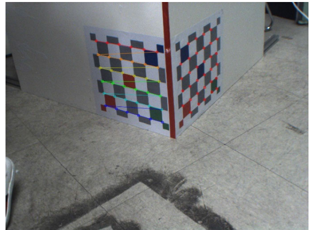
FIGURE 4. Automatically detected control points on the chessboard.
