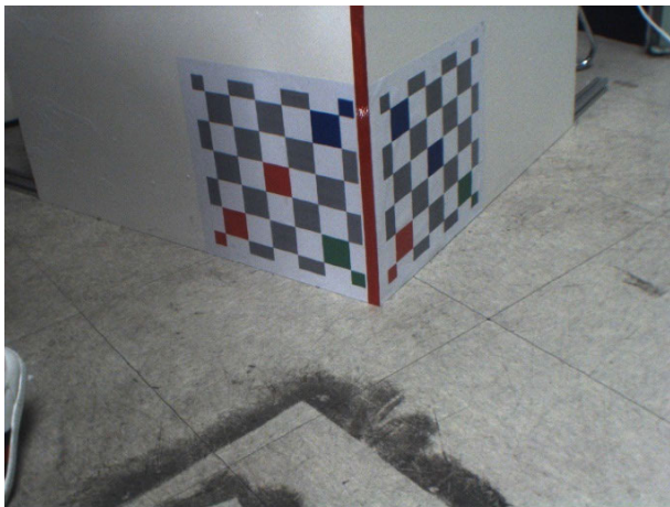
FIGURE 2. Calibration structure with two planes.
