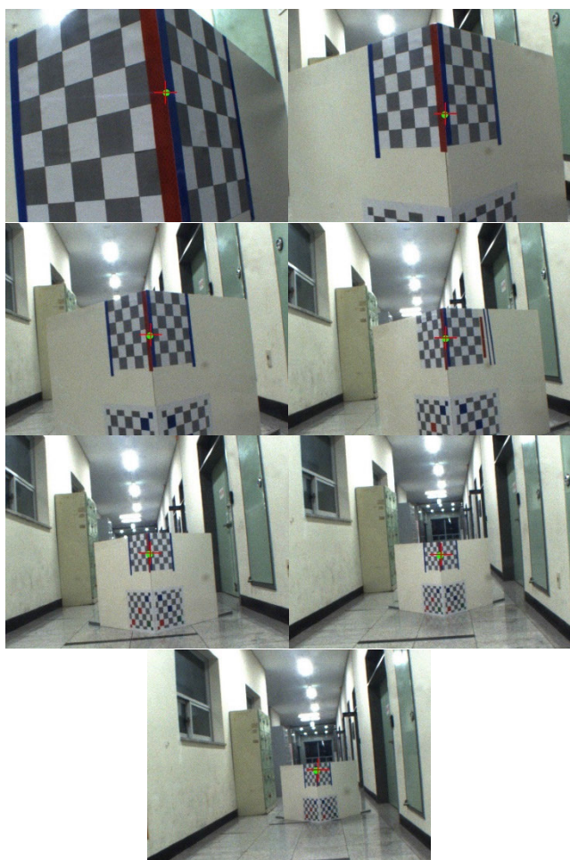
FIGURE 14. Projection results with computed extrinsic calibration on validation sets (green circle is the ground truth, and red cross is the projected point at distances of 0.5m, 1m, 1.5m, 2m, 3m, 4m, 5m).
