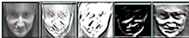
FIGURE 3. Examples of images processed by Gabor wavelet transform with various parameter settings.
