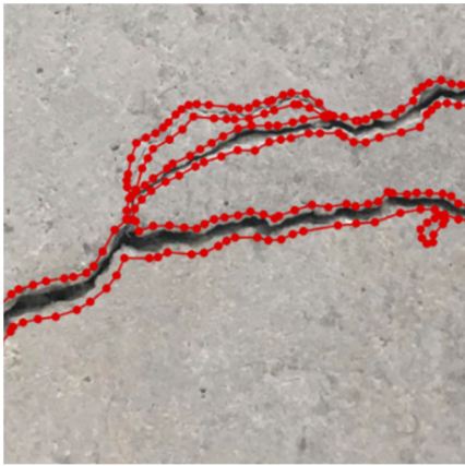
FIGURE 4. Polygonal annotation of images by the authors using LabelMe [57] and used for model training.
