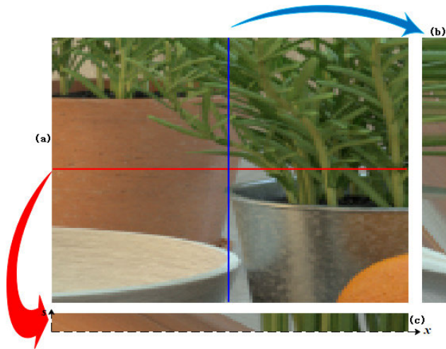
FIGURE 3. EPI examples. (a) is a central view of a light field, and (b) and (c) are EPIs corresponding to the positions of the blue vertical line and the red horizontal line in the central view, respectively.
