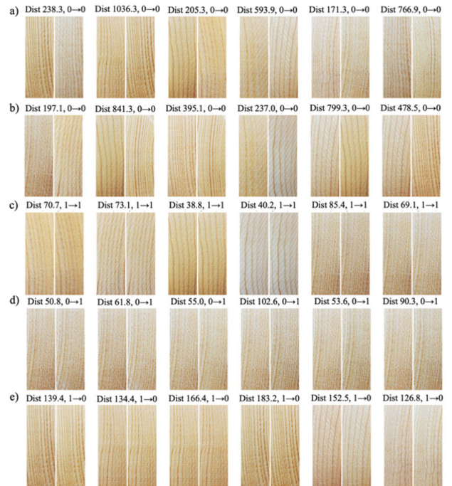
FIGURE 6. Results of recognition on wood biometric images, including correctly recognized a), b), c) and misclassified wood images d), e). The higher label is “ground-truth → prediction”. 1: same, 0: different. Dist: distance.
