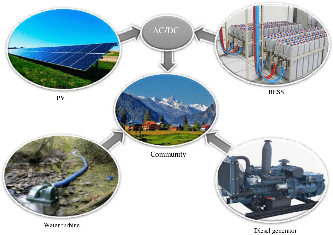
FIGURE 3. The proposed Hy-PV-D-BESS hybrid system configuration.
