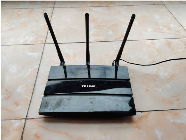
FIGURE 2. The TP-Link WDR4310 router with three antennas used for positioning, with each antenna can receive a set of CSI values of 56 subcarriers.
