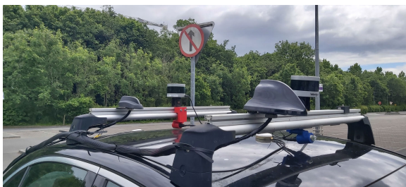
FIGURE 1. Sharkfin antennae mounts on test vehicle.
