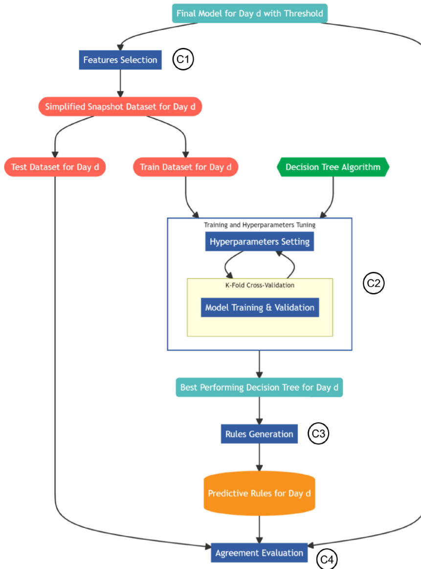
FIGURE 5. Methodology for deriving a collection of prediction rules for model interpretation and knowledge discovery. After computing the Simplified Snapshot Dataset with the most important features extracted by the Features Selection procedure, we train the Best Performing Decision Tree . This model is the result of the training and tuning many Decision Tree models ( Training and Hyperparameters Tuning ) with the aim of finding the best hyperparameters combination for the considered task. From the best performing decision tree, we extract the Predictive Rules via the Rule Generation procedure. Finally, such rules are evaluated in terms of their agreement ( Agreement Evaluation ) with the original model ( Final Generated Model ).
