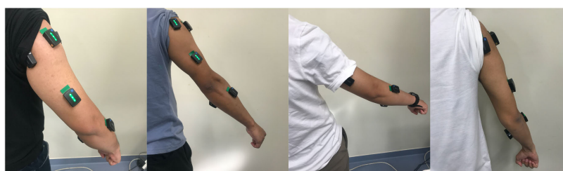
FIGURE 18. Attachment of Delsys EMG sensors in the right hand of subjects.
