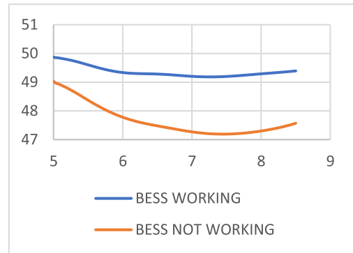
FIGURE 8. Frequency response plot with and without BESS (300 MW load increase).
