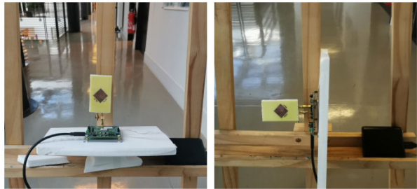
FIGURE 13. Two-way ranging with the designed antenna, characterized by 180° directional radiation and circular polarization.
