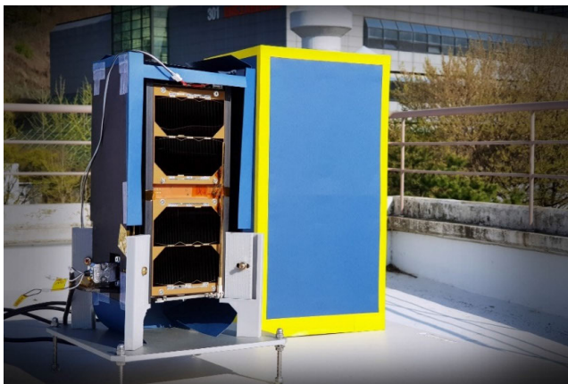
FIGURE 3. Sunscreen and CubeSat cradle for current compensation experiment, which is composed of a screen that exposes one side of the CubeSat and a screen that covers the entire surface.
