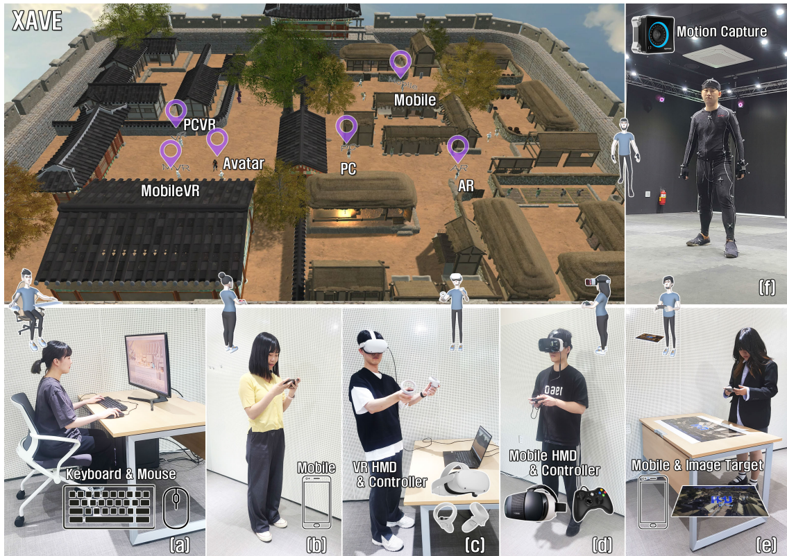
FIGURE 1. Structure of XAVE, a cross-platform based asymmetric virtual environment: (a) PC user, (b) mobile user, (c) PC-based VR user, (d) mobile-based VR user, (e) mobile-based AR user, and (f) actor-based avatar using motion capture.
