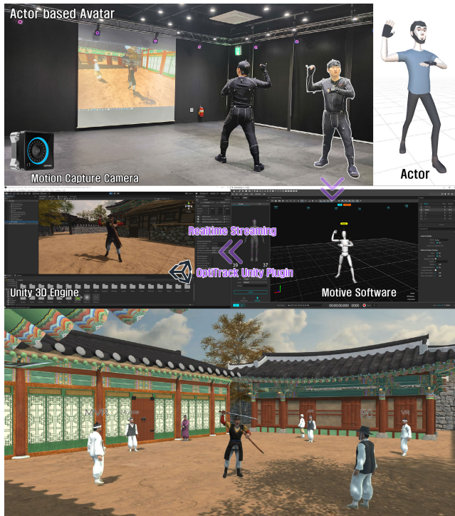
FIGURE 7. Environment set up and data streaming for the construction of actor-based avatar using motion capture.
