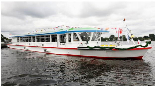
FIGURE 1. The world's first hydrogen fuel cell passenger vessel 'FCS Alsterwasser' [7].
