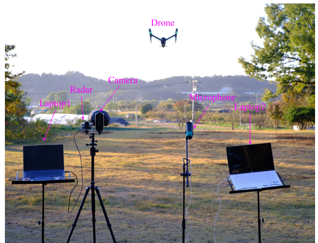
FIGURE 3. Setup for field measurements using the smartphone camera, the FMCW radar, and the microphone.
