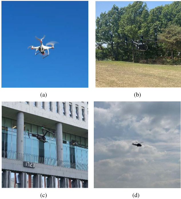
FIGURE 4. Images obtained by the built-in smartphone camera: (a) Phantom4 drone in flight, (b) Inspire2 drone in forest background with a similar color, (c) Inspire2 drone in building background with a similar color, (d) Military helicopter.
