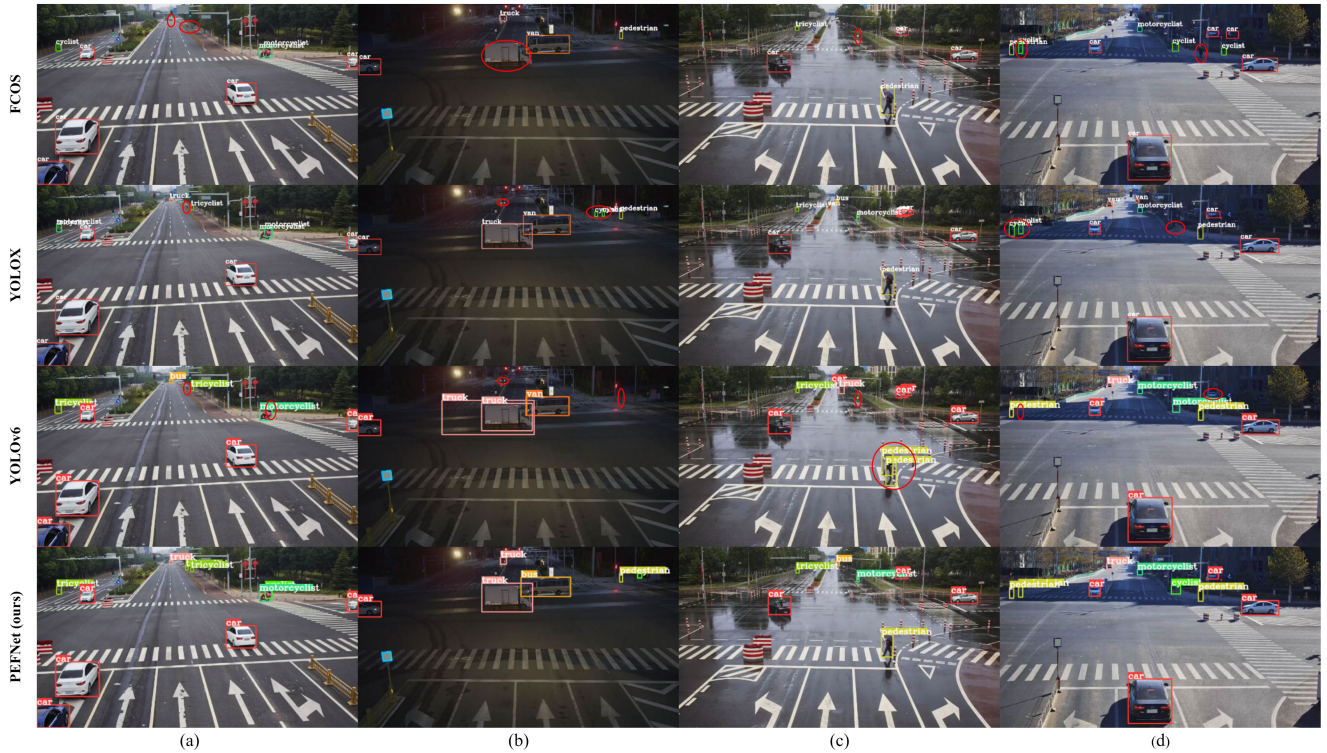
FIGURE 15. Comparison of roadside detection in different scenarios captured by roadside visual sensors (Rope3D dataset). Cases of missed detection and false detection are highlighted in red.
