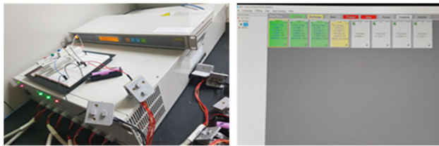
FIGURE 14. The experimental testbed was used to collect custom datasets with the lithium-ion battery INR-18650 for evaluating the proposed SOH prediction and anomaly detection system.
