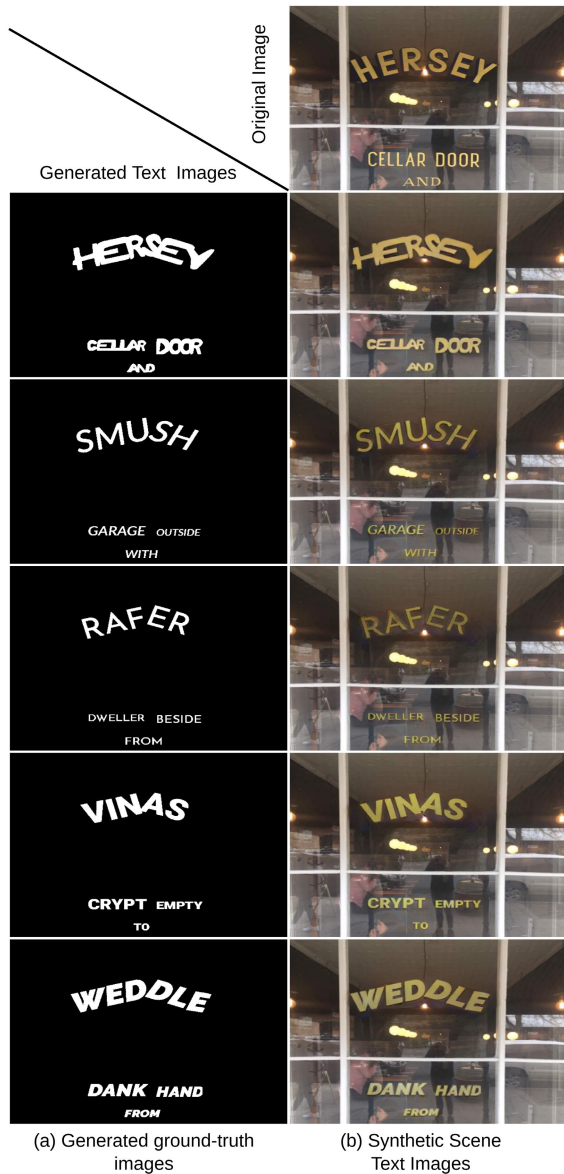
FIGURE 1. Results of paired synthetic data on the training set. The generated text images (a) from the proposed text image generator have different words and fonts. The original image is from the public scene text image dataset. With one given original image and the different text images, the proposed GANs can generate different scene text images naturally (b). As a result, we have new paired data (scene text image and text segmentation ground truth) for the scene text segmentation task.
