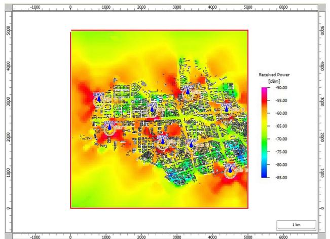
FIGURE 5. The coverage effect of 8 UAVs based on COST231-Hata model in Haidian island, Haikou city. The global utility is 59.49%.
