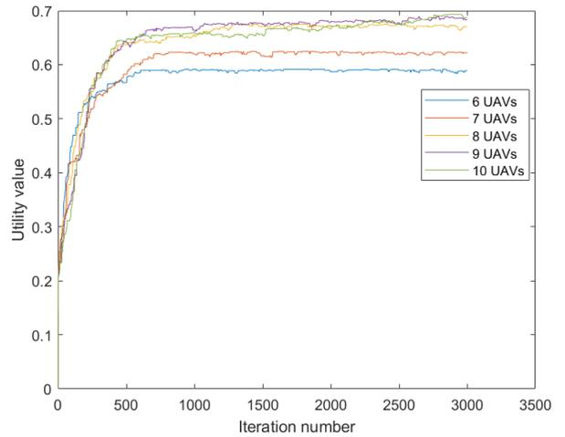
FIGURE 9. The iterations of 6-10 UAVs: it shows proposed method can achieve stable iterative results.
