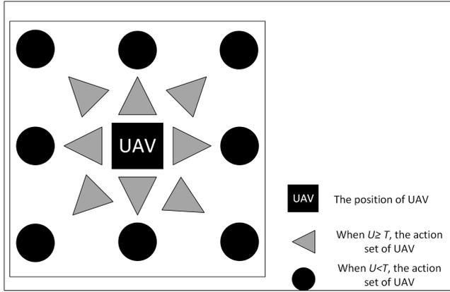
FIGURE 2. The action set: it has two different motion sets to be chosen.
