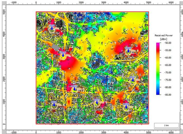
**FIGURE 11.** The coverage effect of 8 UAVs based on COST231-Hata model in Guangzhou. The global utility is 62.76%.
