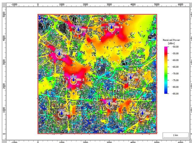
**FIGURE 13.** The coverage effect of 8 UAVs based on log-distance model in Guangzhou. The global utility is 63.99%.
