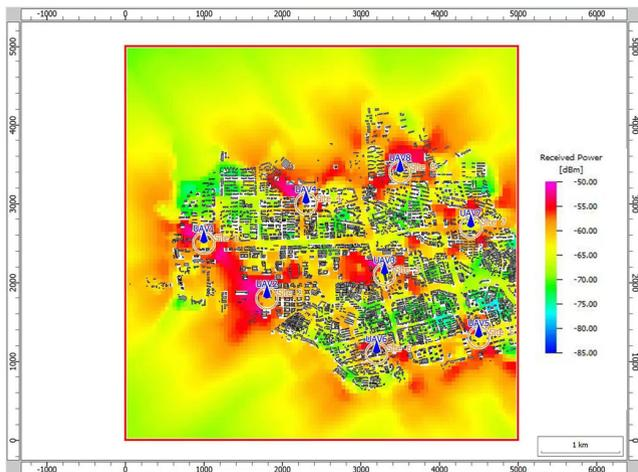
FIGURE 7. The coverage effect of 8 UAVs based on log-distance model in Haidian island, Haikou city. The global utility is 60.01%.
