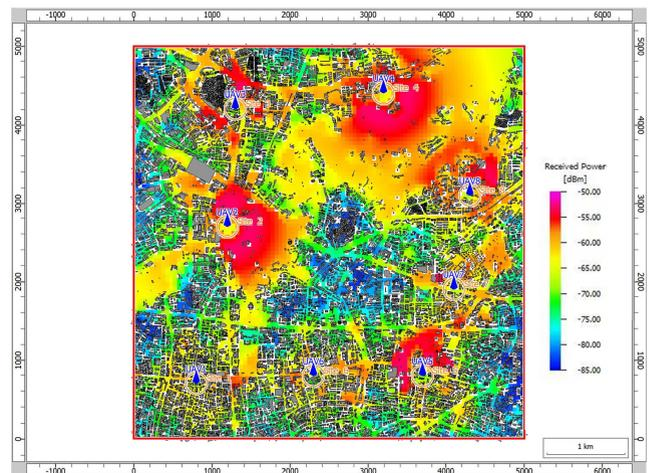
FIGURE 10. The coverage effect of 8 UAVs based on RF model in Guangzhou. The global utility is 63.60%.
