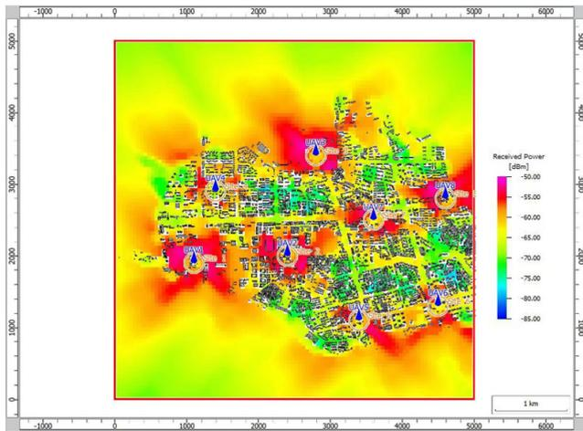
FIGURE 6. The coverage effect of 8 UAVs based on FS model in Haidian island, Haikou city. The global utility is 58.70%.
