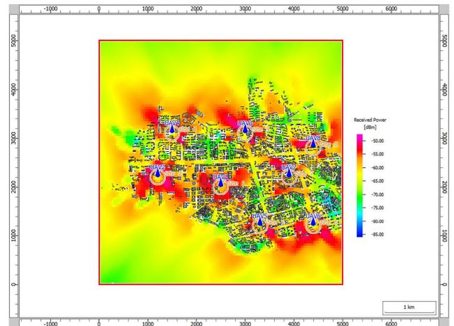
FIGURE 4. The coverage effect of 8 UAVs based on RF model in Haidian island, Haikou city. The global utility is 60.07%.
