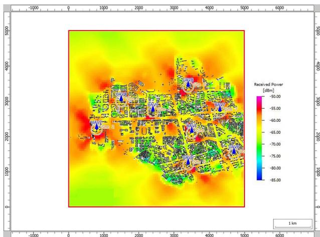
FIGURE 8. The coverage effect of 8 UAVs based on ray-tracing method in Haidian island, Haikou city. The global utility is 68.27%.
