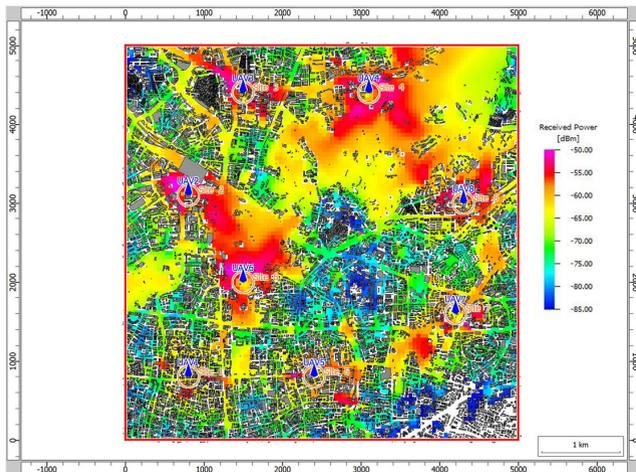
**FIGURE 12.** The coverage effect of 8 UAVs based on FS model in Guangzhou. The global utility is 62.64%.
