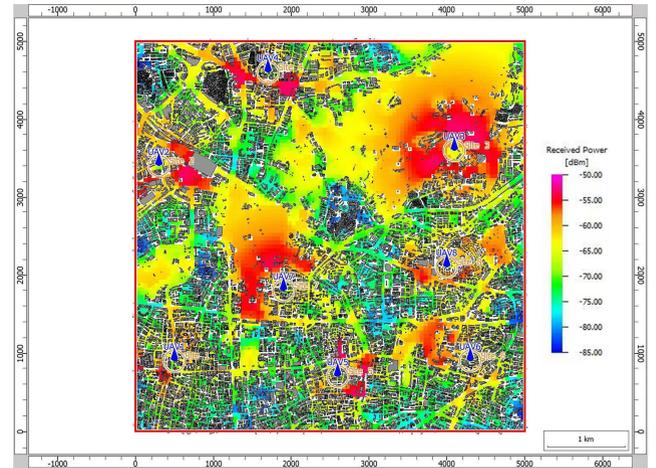
**FIGURE 14.** The coverage effect of 8 UAVs based on ray-tracing method in Guangzhou. The global utility is 68.78%.
