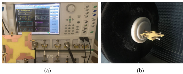
FIGURE 17. Scattering parameters, radiation pattern, and gain measurement setup: (a) Measurement setup for scattering parameters of the quad-port MIMO dipole antenna, (b) Measurement setup for radiation pattern and gain of the quad-port MIMO dipole antenna.
