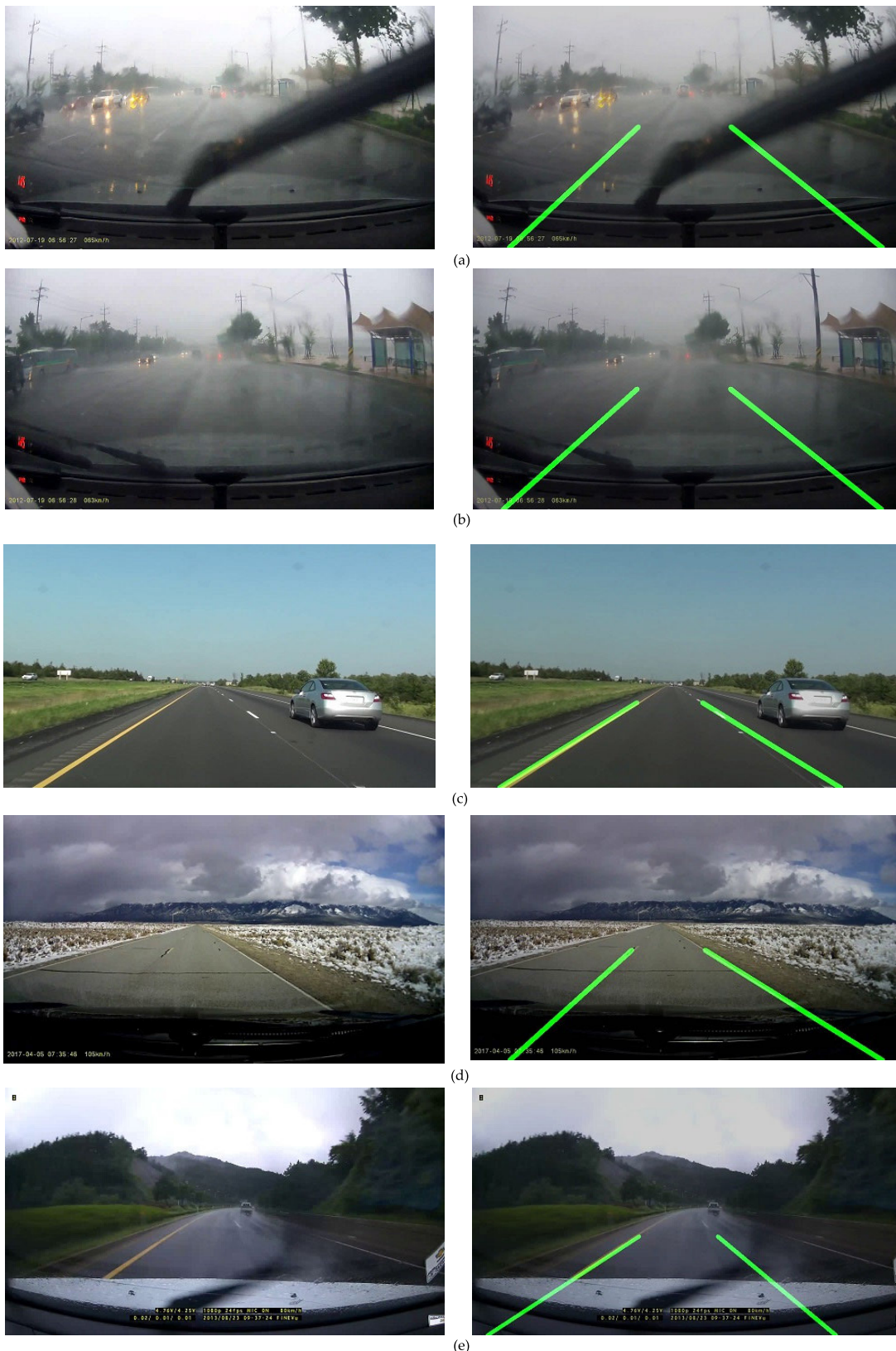
FIGURE 10. Successful lane detection and tracking under different challenges from DSDLDE dataset; (a) both lanes are eroded and right lane is occluded by wiper, (b) unpainted road, (c) right lane is dashed and slightly eroded, (d) left lane marking is cracked and fully eroded (e) right lane is dashed, blurred due to rain and occluded by wiper (f) both lane is almost eroded and fully invisible due to white out tunnel exit (g) left lane is invisible due to darkness and overexposed headlight reflection on windshield (h) right lane is invisible due to shiny effect created by street lamp and taillight reflection on wet windshield.
