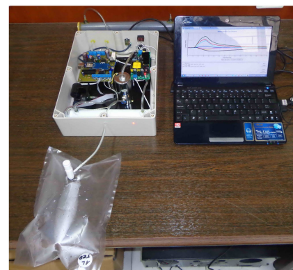
FIGURE 2. Electronic nose used in experiment: (a) block diagram, (b) realization.
