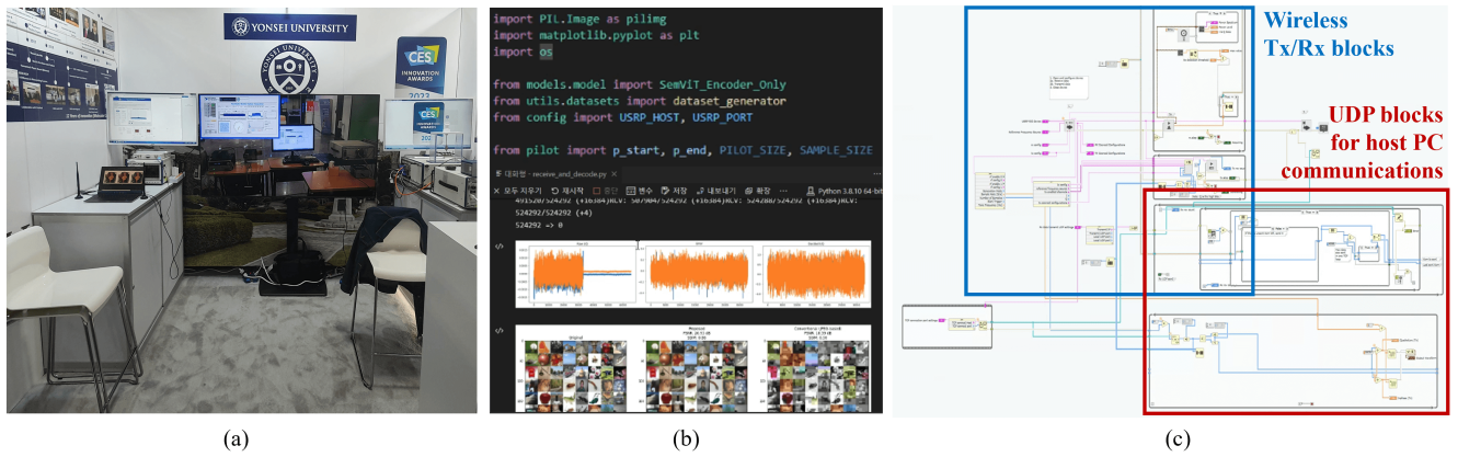
FIGURE 9. (a): Real-time demonstration of the proposed system in a crowded indoor environment (at CES 2023, Las Vegas, USA), (b) screenshots of the client/server (for neural encoding/decoding), and (c) the LabVIEW block diagram (for real-time wireless transmission). Both softwares, including neural network parameters, are available open-source. See https://bit.ly/SemViT/ .
