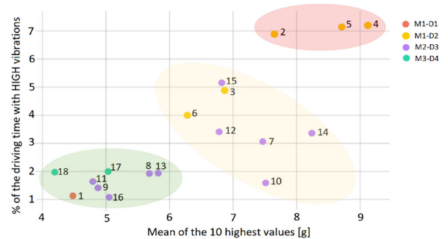
FIGURE 14. Scatterplots of the centroids for particular haul trucks (including mining departments). Measures calculated for the Z-axis accelerometer located in the working unit.
