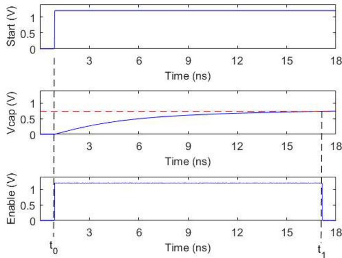
FIGURE 6. Example of operation of the circuit where the capacitor ( $cap=10$  fF) starts charging at  $t_0$  and  $V_{cap}$  reaches the threshold value after  $17.2$  ns ( $t_1$ ) for  $R_{HRS} = 1.52$  k $\Omega$ . The Enable signal of the counter is active during the ( $t_0, t_1$ ) interval.
