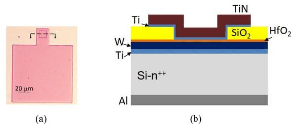
**FIGURE 1.** The RRAM devices used in this study (a) Top view image. (b) The cross sectional schematic.
