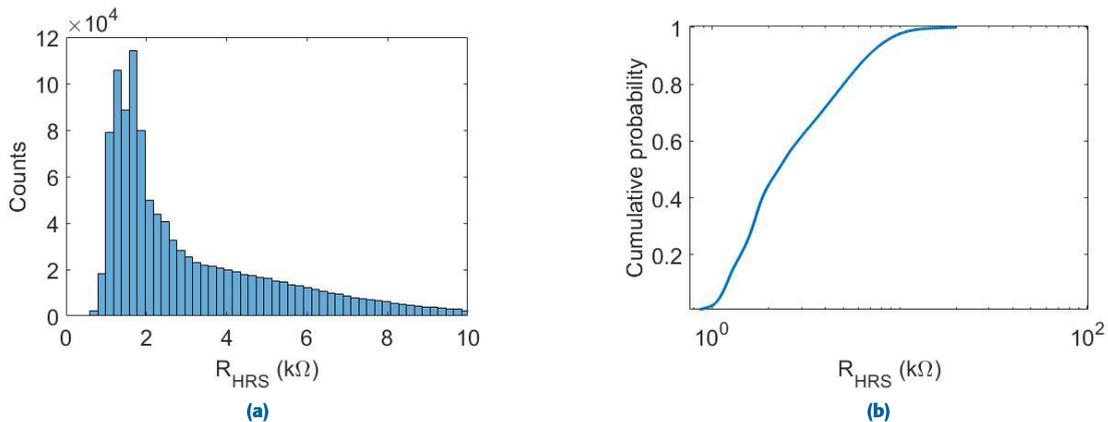
FIGURE 4. (a) Distribution of the experimental  $10^6 R_{HRS}$  measured values from a sample RRAM under pulsing operation. The experimental data follow a lognormal distribution with  $\mu=7.86$  and  $\sigma=0.65$  (b) Cumulative probability plot.
