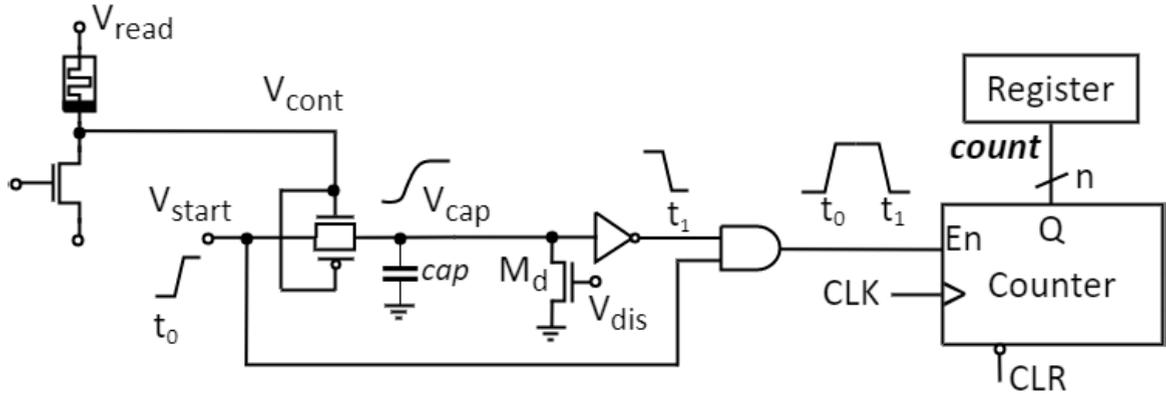
FIGURE 5. Circuit for converting the  $R_{HRS}$  value into a delay with n-bits resolution.
