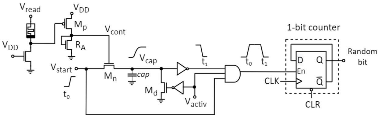
FIGURE 7. Circuit for the generation of one random bit by means of one RRAM device.
