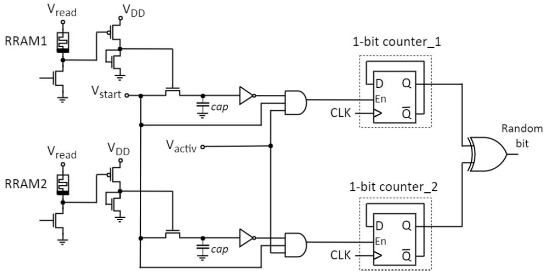
FIGURE 10. Circuit for the generation of one random bit by means of two RRAM devices.
