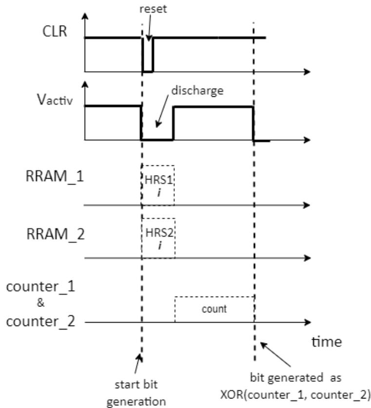
FIGURE 11. Reset and active signals during the process of generating a random bit by means of two RRAMs. Each HRS cycle is preceded by a LRS not shown in the time diagram.
