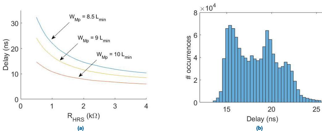
FIGURE 9. (a) Delay dependence on  $R_{HRS}$  for different widths of pMOS transistor  $M_p$ . (b) Distribution of delays.
