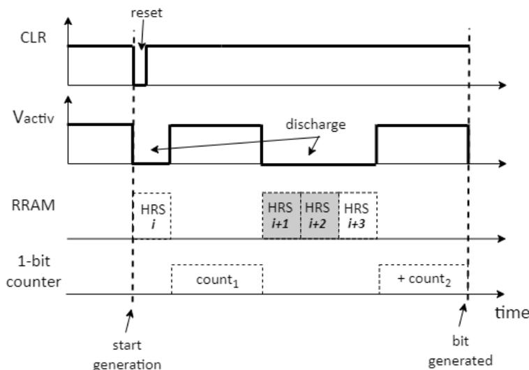
FIGURE 8. Reset and active signals during the process of generating a random bit. Note that each HRS cycle is preceded by a LRS not shown in the time diagram. Dummy HRS cycles are indicated in grey.
