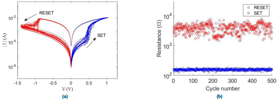
FIGURE 3. (a) Current/Voltage characteristics of the RRAM during successive SET and RESET operations in DC mode. (b)  $R_{LRS}$  and  $R_{HRS}$  resistances after SET and RESET operations in pulse mode.
