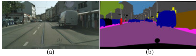
FIGURE 1. Labelling class to each pixel in semantic segmentation. (a) Original input image, (b) colored annotation of the input image where each pixel of the image has a specific color code.
