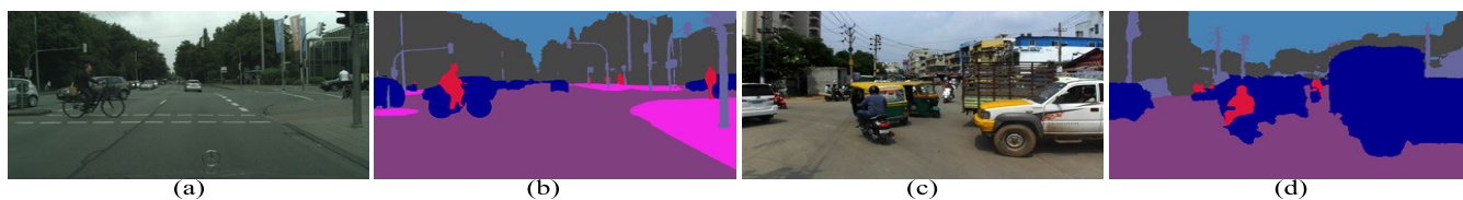
FIGURE 17. Models predictions using Cityscapes and IDD samples on 7 classes. (a) Cityscapes input, (b) Cityscapes prediction, (c) IDD input, (d) IDD prediction.
