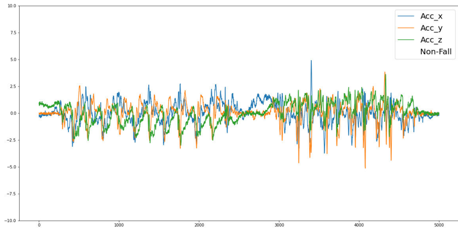
(a) 3-axis accelerometer signals during walking upstairs at a slow pace.
