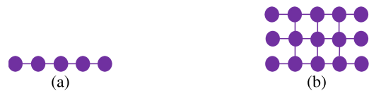
FIGURE 3. Cluster states generation and preparation (a) 1D cluster state. The circles represent qubit states and the line between two circles represents the controlled-phase operation between the corresponding qubits. (b) 2D cluster state.
