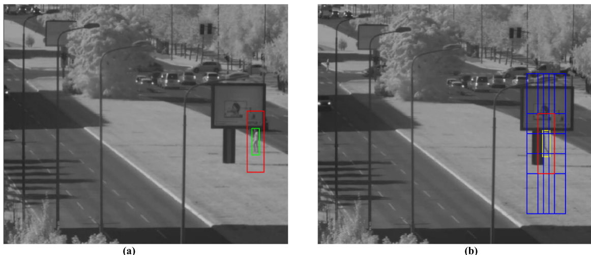
FIGURE 4. a) Object tracking in the regular conditions using a single search window (--- tracked object, --- search window) b) Multiple search windows are activated after the failure is detected (--- estimation of tracked object, --- central search window predicted by the Kalman filter, --- surrounding 8 overlapped multiple search windows).
