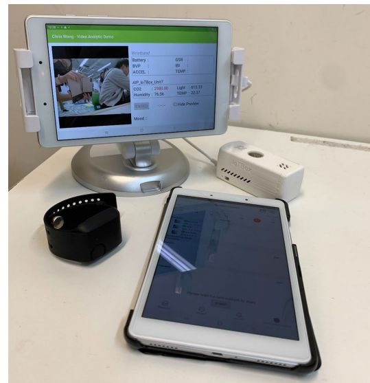
FIGURE 2. Perception layer equipment set of the current study. It includes an Empatica E4 wristband (left), a IoT sensors box with SoC controller (right), an edge tablet PC for assessment labels input (bottom), and a display screen of real-time data (top).
