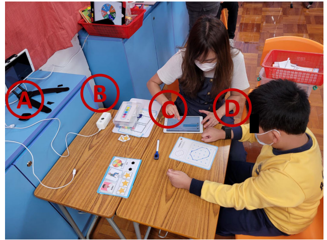
FIGURE 5. The setting of an ABA session in our study. (A) A screen display shows various real-time data related to the ABA session recommended by the 3I-Learning System. (B) An IoT sensors box contains environmental sensors. (C) An assessment interface records the therapist’s task analysis results in real-time. (D) An Empatica E4 wristband collects the student’s physiological and motion data.
