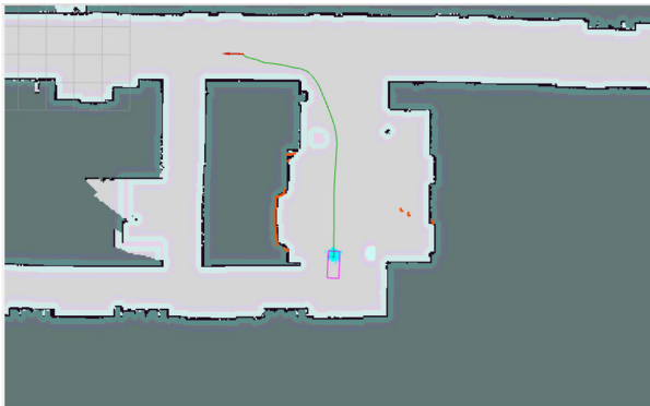
FIGURE 14. Path planning result when the user is guided to avoid colliding with a chair by proposed potential field method considering spatial risk map.
