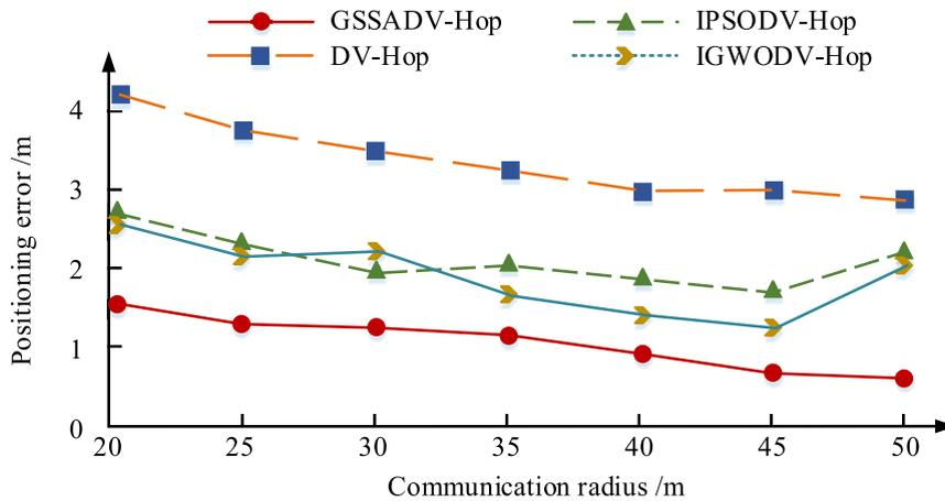
FIGURE 9. Positioning error influenced by communication radius.
