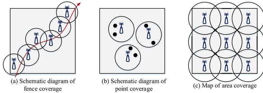
FIGURE 1. Schematic diagram of different types of WSN coverage.
