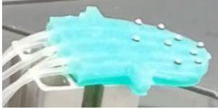
FIGURE 10. The nine markers on the robotic tongue surface.
